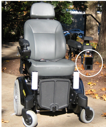
Figure 1: Prototype smart wheelchair system integrating the the flash LIDAR (encircled white).
